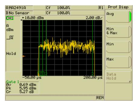
Figure 3. 802.11a Burst with 2 gates applied
