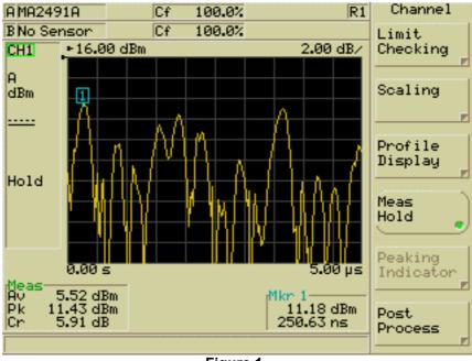
Figure 1. Power Envelope of a WCDMA transmission
