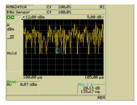
Figure 4. A view of 5µs of the data payload in a 802.11a,OFDM, 64QAM, 54Mb/s signal
